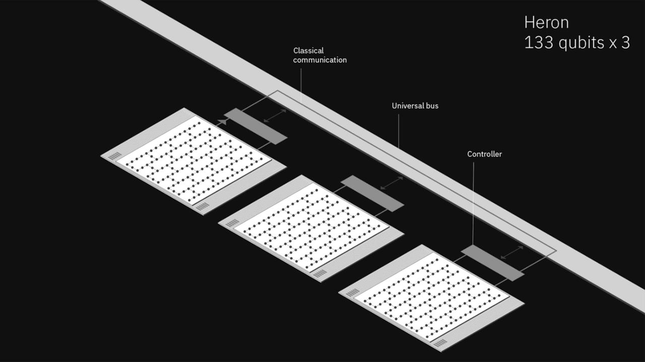
Quantum communication via two qubit gates between separate chips
